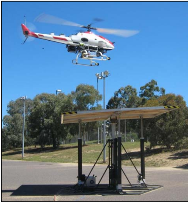
FIGURE 9. UNSW@ADFA R-Max hovering over moving deck simulator.
