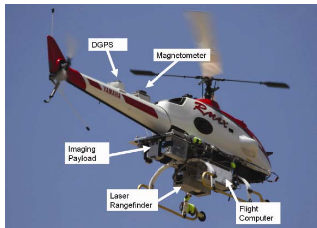
FIGURE 1. UNSW@ADFA R-Max in flight during laser-rangefinding experiments
